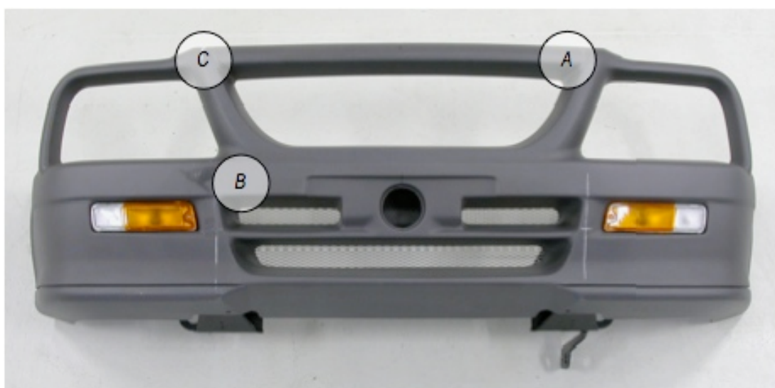
Figure 3.14 Holden Rodeo aftermarket polymer bull bar test locations. Letters correspond to test locations for Part A, B and C tests
