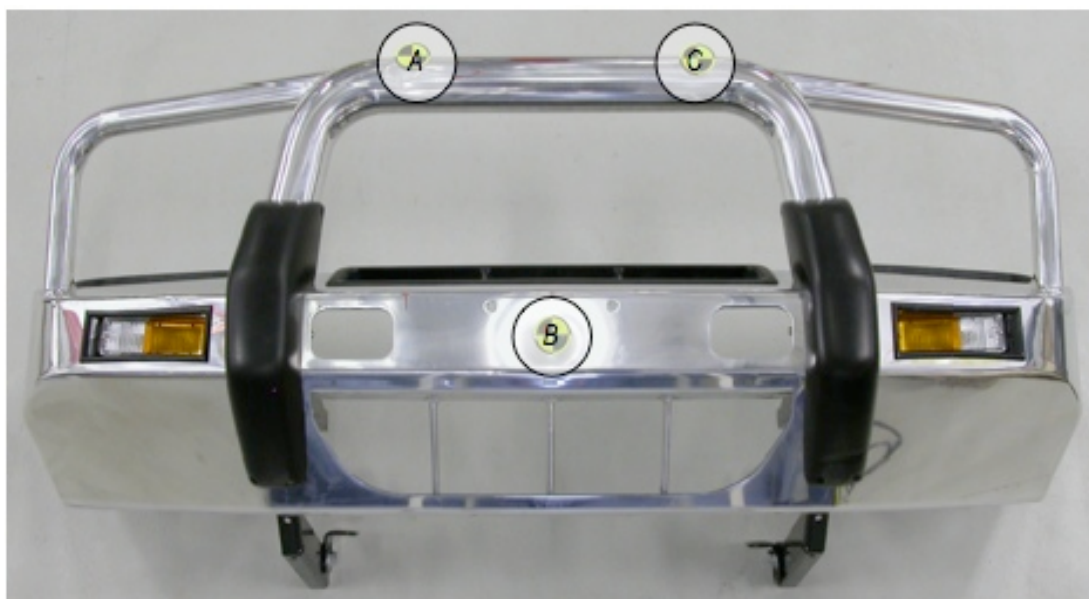
Figure 3.10 Ford Courier OES alloy / aluminium bull bar test locations. Letters correspond to test locations for Part A, B and C tests
