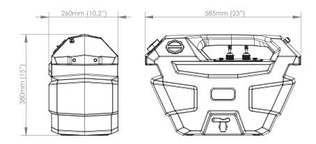
Tank Weight: Empty - 4.5kg (9.9lb) Filled with water + soap - 32.5kg (73.9lb) **Volume:** 28L (7.4 gal)
