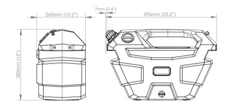
Tank Weight: Empty - 4kg (8.8lb) Filled with diesel -34kg (73.9lb)
